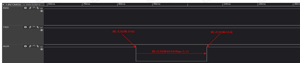
Hardware mode switching AUX timing
